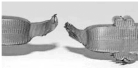
(b) Ductile Rupture Outside Fusion Interface
